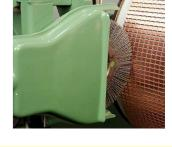
Removes the sharp edges on undercut copper bars while creating a smooth radius on the corner of the bar. Works in minutes. Eliminates hours of hand scraping.
