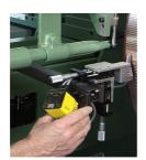
Fiber optic sensor automatically identifies the mica slot to align the saw.
