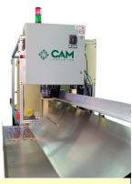
Stainless steel accumulation table protects finished wire from contamination.
