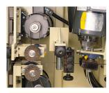
Special angled brushes automatically strip away the insulation cover without damaging the copper wire.
